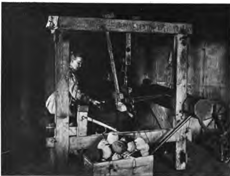
HAND-LOOM AND SPINNING-WHEEL FOR FLAX.
